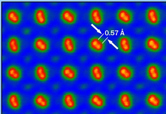
Double Yttrium columns resolved in an HAADF STEM image of a YAP crystal. Alternate double columns have different orientations. Nion UltraSTEM™, 200 keV. Courtesy Dr. M.F. Chisholm, ORNL, and SMRC, U. Tenn.
