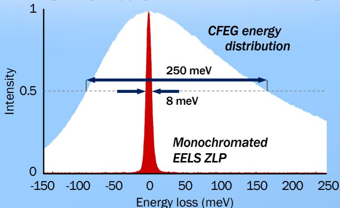
Zero loss peak (ZLP) acquired with Nion UltraSTEM-MC™, 8 ms, 60 keV primary voltage, compared to the unmonochromated ZLP. Courtesy Rutgers U.
